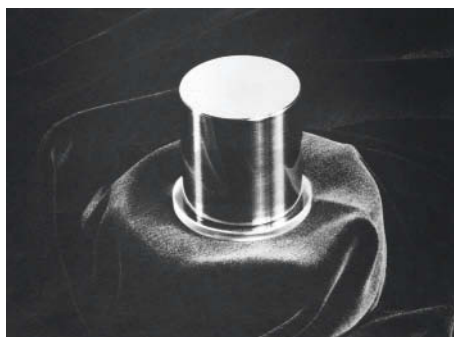
FIGURE 1.2 The standard platinum–iridium kilogram is kept at the International Bureau of Weights and Measures in Sèvres, France. This copy of it was assigned to the United States in 1889 and is housed at the National Institute of Standards and Technology.
